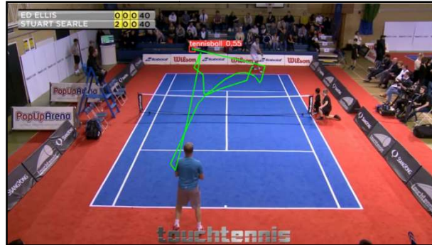
Figure 18 The images that detect the position of tennis balls have some inaccuracies
