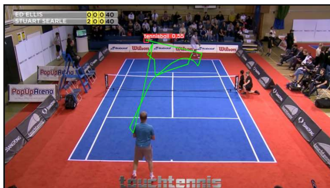
Figure 23 The images that detect the position of tennis balls have some inaccuracies
