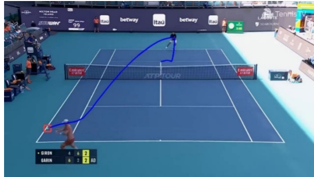
Figure 26 Detecting tennis balls using deep learning and Kalman filter of frame 48
