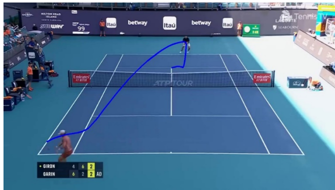
Figure 28 Detecting tennis balls using deep learning and Kalman filter of frame 50
