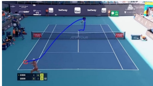
Figure 25 Detecting tennis balls using deep learning and Kalman filter of frame 47
