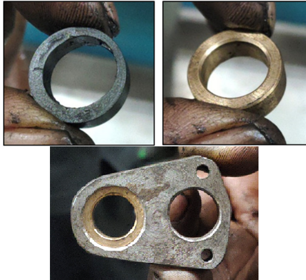
Figure 7 Plastic bushing is deteriorate (left) brass bushing (right) Ready-assembled brass guide bushings (bottom)
