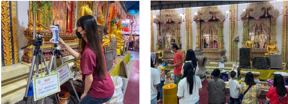
Figure 2 Show of RD sampling by Personal air sampler pump and PM 2.5 sampling by Indoor air quality monitor.
