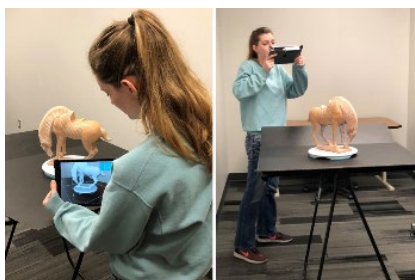
Figure 3: Scanning using the Occipital Structure Sensor
