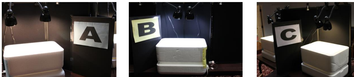
Figure 6. Three lighting treatments (LED - warm, LED - cool and compact fluorescent,) illuminating raw ground beef packages in styrofoam ice chests
