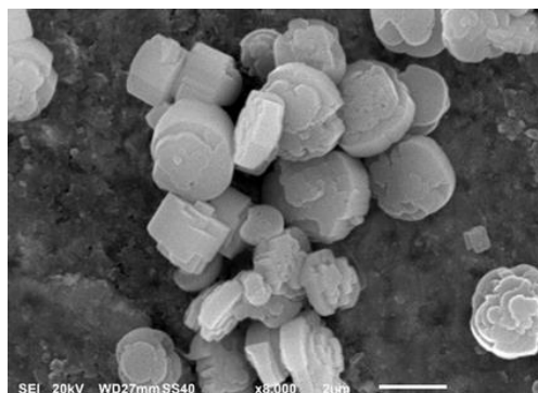
Figure 2 Scanning electron microscopy images of Zeolite KLTL at 8,000 \times magnification
