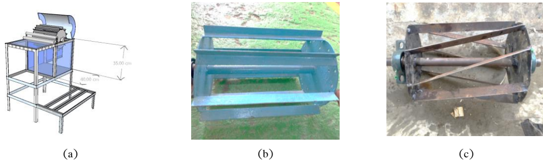
Figure 1 This is the fiber separation machine: (a) Machine design (b) 0° blade angle (c) 15° blade angle
