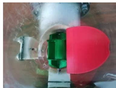
Figure 3 Guide vane (red colour)
