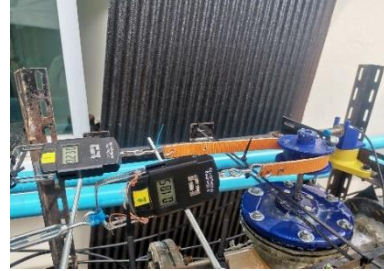
Figure 7 System to measure the torque of the hydro turbine
