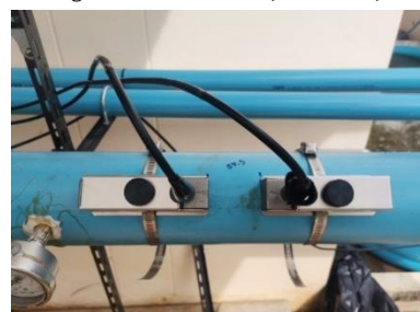
Figure 5 Flow Sensor positioning
