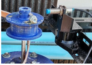
Figure 6 Proximate sensor to measure the speed of the turbine
