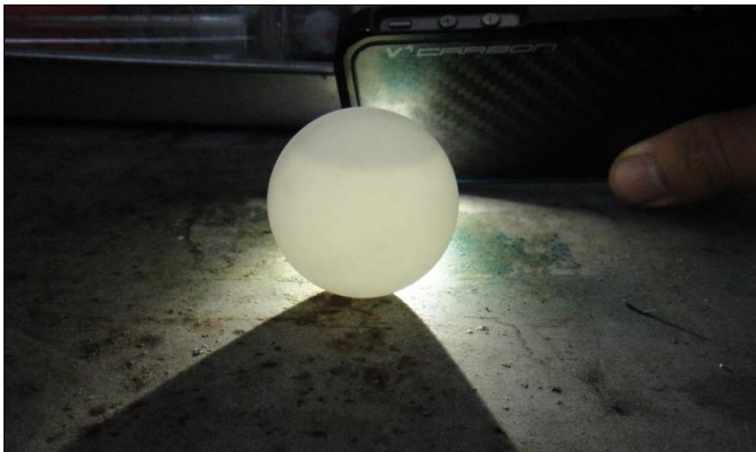
Figure 2 The PCM ball used in the PCM bed.
