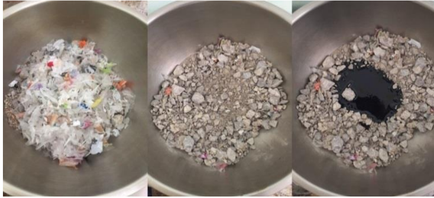
Figure 2 The laboratory mixture of plastic bag waste with para-asphalt concrete (left: added shredded plastic bag waste to aggregate; center: mixing shredded plastic bag waste with aggregate; right: added para-asphalt cement to mixture)
