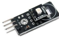
Figure 3 UVM-30A UV sensor module
