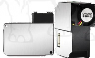
Figure 5 PMS-3003 sensor module.
