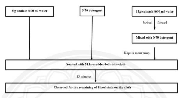
Figure 3 Diagram of experimental methods
