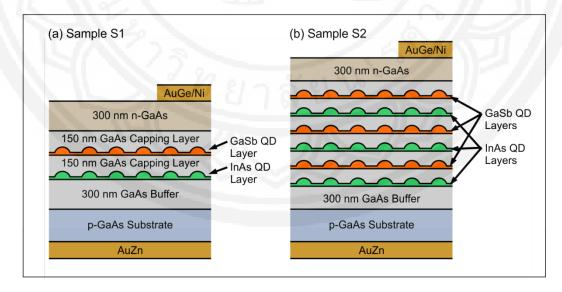
**Figure 1** Schematics of investigated hybrid QD solar cell samples. The sample (a) S1 and (b) S2 have one pair and three pairs of stacked InAs/GaAs QD and GaSb/GaAs QD layers, respectively
