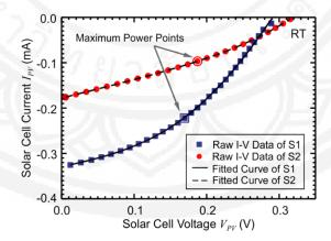
**Figure 3** Current-voltage characteristic curves of sample S1 and S2. Raw experimental data of sample S1 and S2 are shown in blue squares and red circles, respectively. The solid and dashed lines are the fitting results according to the applied DC equivalent circuit model. Maximum power points of each data are marked
