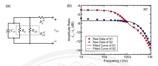
**Figure 5** (a) AC equivalent circuit of hybrid QD solar cell and (b) frequency responses of the hybrid QD solar cells biased at maximum power points (marked in Figure 3). Amplitude ratio  $A_{out}/A_{in}$  obtained from the samples S1 and S2 are plotted with blue squares and red circles, respectively. The solid and dashed lines are the fitting with the AC equivalent circuit model shown in (a)
