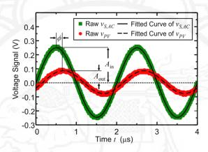
Figure 4 Waveforms of AC biased voltage  $v_{S,AC}$  and solar cell voltage  $v_{PP'}$  (of sample S1) obtained at the frequency of 500 kHz. The sample is DC biased at the maximum power point. Input and output amplitudes  $A_{in}$  and  $A_{out}$  as well as the phase difference  $\phi$  are extracted by the fitting with sinusoidal functions as shown as solid and dashed lines
