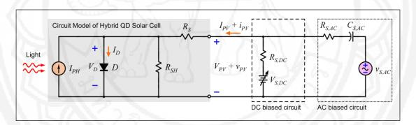
Figure 2 Circuit diagram for both DC and AC parameter extraction. The DC biased circuit is shown in the dashed frame and the AC biased circuit is shown in the dotted frame. The shaded area contains DC equivalent circuit model of hybrid QD solar cell
