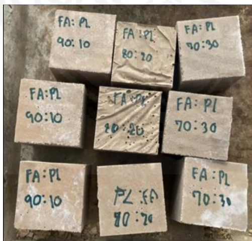
(a) after exposed to 500°C
