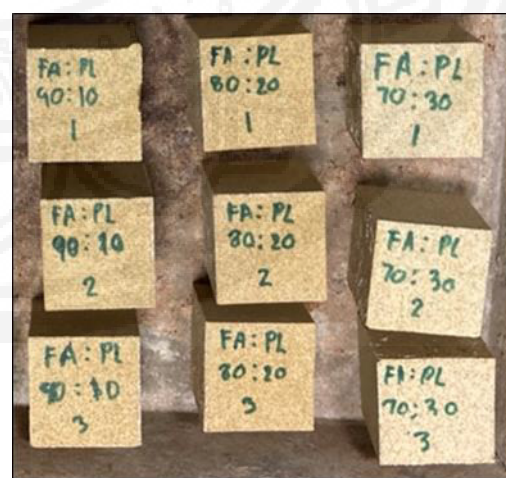
(b) after exposed to 1000°C
