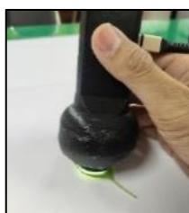
Figure 7 Pesticide residues scanned by using the proposed portable spectrometer
