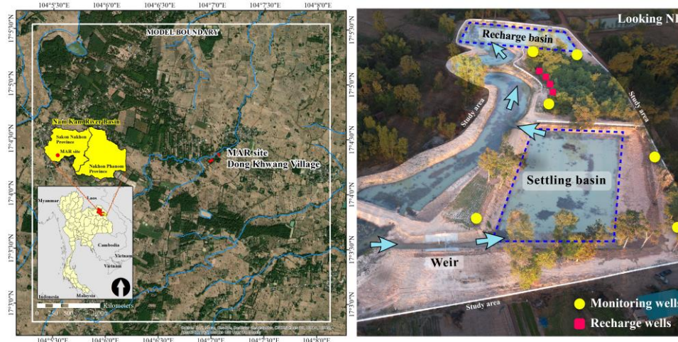
Fig. 3: (Left) A map showing a location of the pilot MAR trial. (Right) An aerial photo of the study area illustrating the system components.
