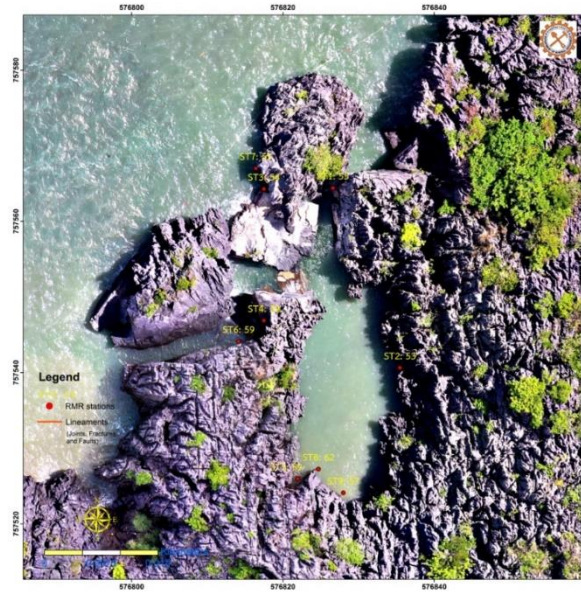
Fig. 7 showing stations of measured Rock Mass Rating overlying on orthophoto
