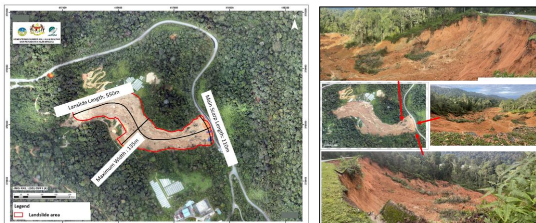
Fig. 3: Dimension of the landslide and the photo of the main landslide body.
