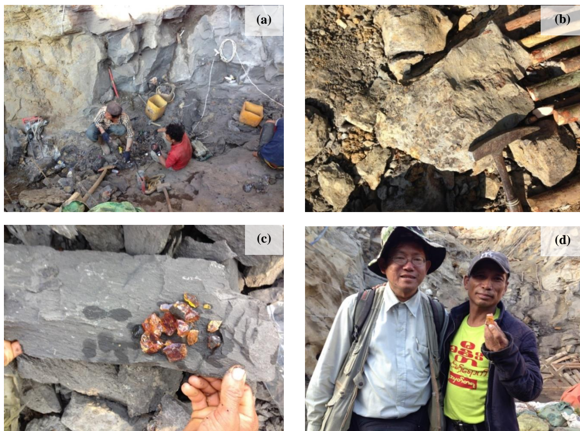
Fig 5: Amber excavation at Laychun Maw: (a) Manual extraction of amber by manpower outside of the adit; (b) amber with carbonaceous materials in limestone; (c) extracted amber and (d) yellowish brown honey colour amber from Laychun Maw. (photos by Thet Tin Nyunt)
