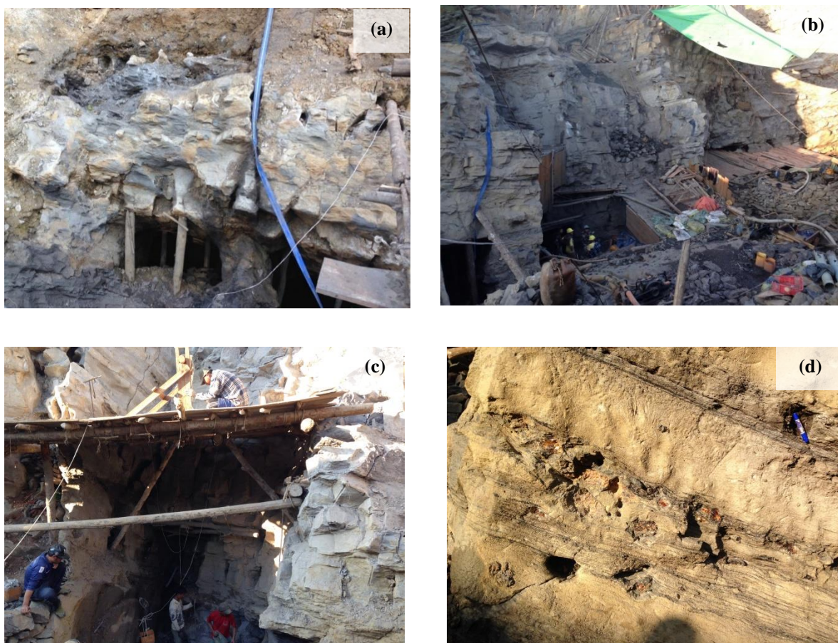
Fig. 6: Nature of amber bearing limestone and amber production at Laychun Maw: (a-b) Entrance for adit of the amber bearing limestone along the bedding plane where the amber is obtained; (c) The amber from amber bearing limestone is transported by a pulley system (yellow bucket with rope and pulley); (d) Intercalation of amber bearing limestone and carbonaceous materials, sometimes with sandstone. (photos by Thet Tin Nyunt)
