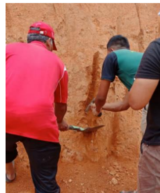
Fig. 4: Sampling of weathered bedrock.
