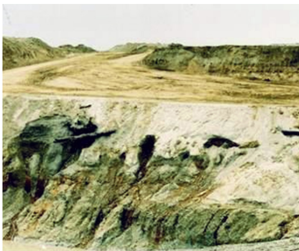
Fig. 100: Early operation of open pit Bo Phloi gem mine western Thailand with yellow sands (loess) on top and numerous burnt felled trees on gravels with sapphire grains.
