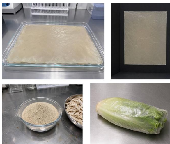
Figure 1 Oyster mushroom powder, bio-film, and wrapped vegetable sample used for sensory evaluation of freshness and crispness
