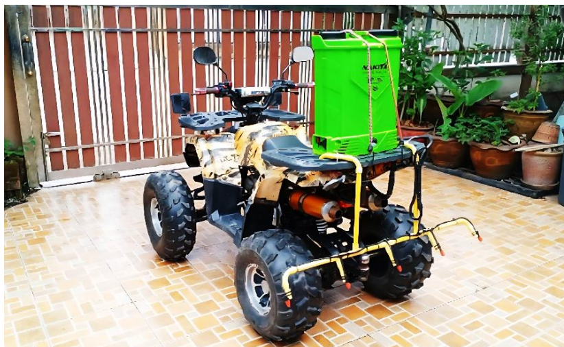
Figure 4 Trailer herbicide sprayer for community enterprises in large agricultural areas
