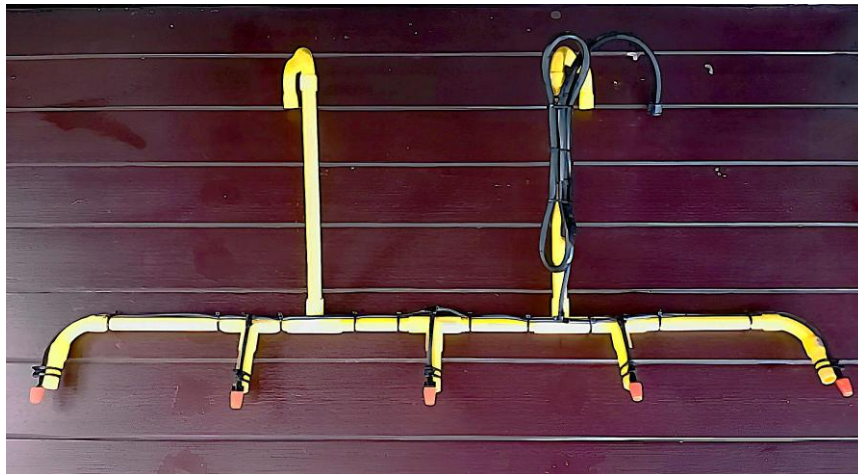
Figure 1 Structure of the trailer sprayer boom
