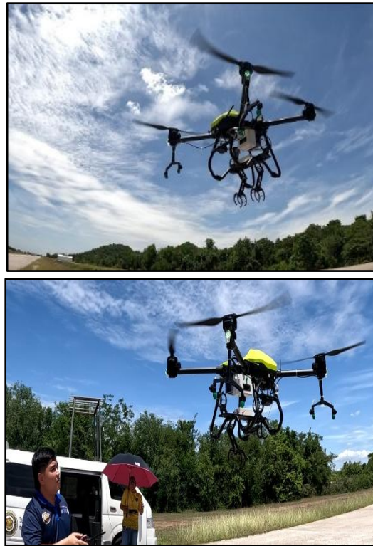
Figure 2 Actual field flight testing of the robotic arm-equipped UAV
