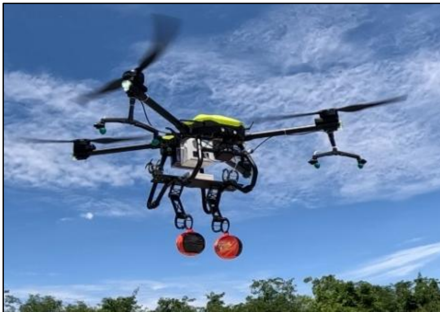
Figure 1 Gripper holding a fire extinguishing ball
