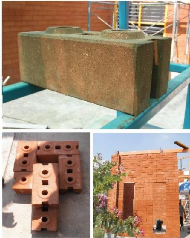
Figure 2 General interlocking block
