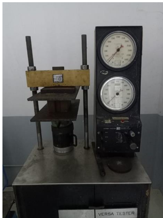
Figure 5 Compression test of interlocking block
