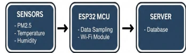
Figure 1. Block diagram of the proposed IoT-based environmental monitoring system.
