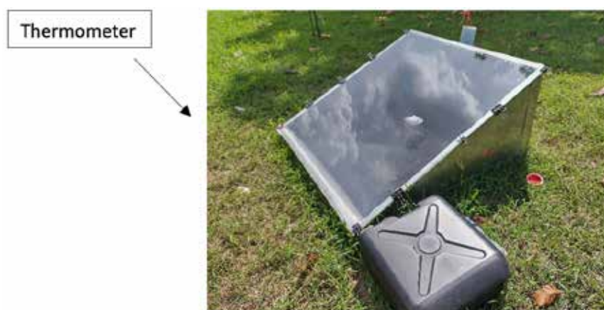
Figure 5 The prototype solar still was tested for water recovery and treatment of brine water from a small-scale desalination. Digital thermometer was placed inside (arrow).
